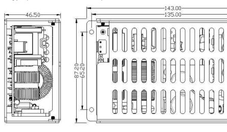
Dimension: L143xW 87.2xH46.5mm Tolerance +/-1mm
