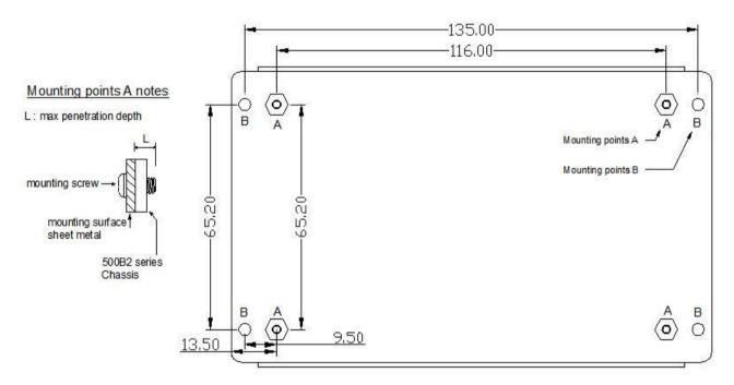
Mounting points A, M3X0.5 thread, Max. Penetration depth (L) 2.5mm.
