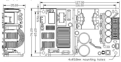
Dimension: L127xW76.2xH35mm Tolerance +/-1mm
