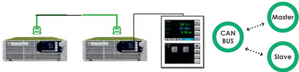
Through a simple and fast setup, the VPG-L series can generate higher power by connecting identical models in a Master/Slave parallel operation. Users only need to control the master unit for multiple units' setup and readbacks. The master unit automatically calculates the parameters and downloads data to slave units to make programming easier and current sharing more precise.
