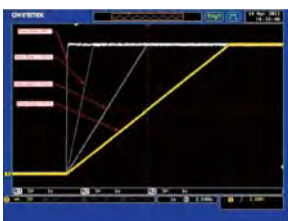
The Adjustable Rise Time of the PSW 30V
