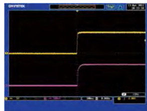
The CC Priority Feature Effectively Limits the Occurrence of Inrush Current and Surge Voltage when the Supplied Voltage Rises to the LED Forward Voltage
