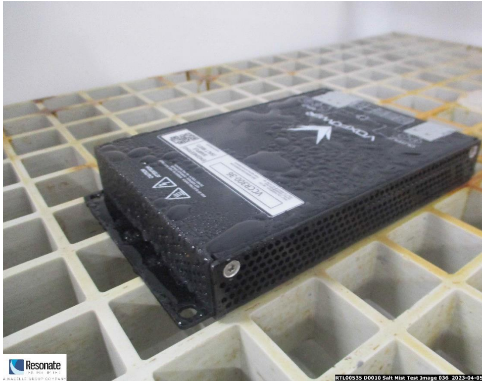
Figure 7: 24-hour fallout check -VCCR300-36
