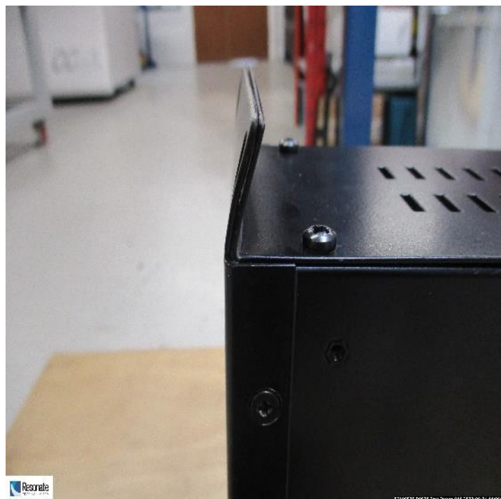
Figure 10: Observation after drop 4, Face 4, bending on front plate
