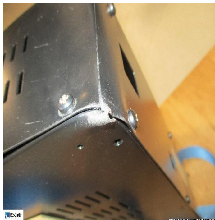
Figure 16: Observation after drop 19, damage on impact edge
