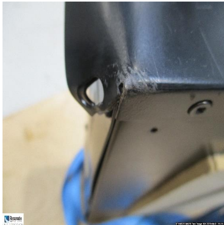
Figure 17: Observation after drop 23, Corner damage
