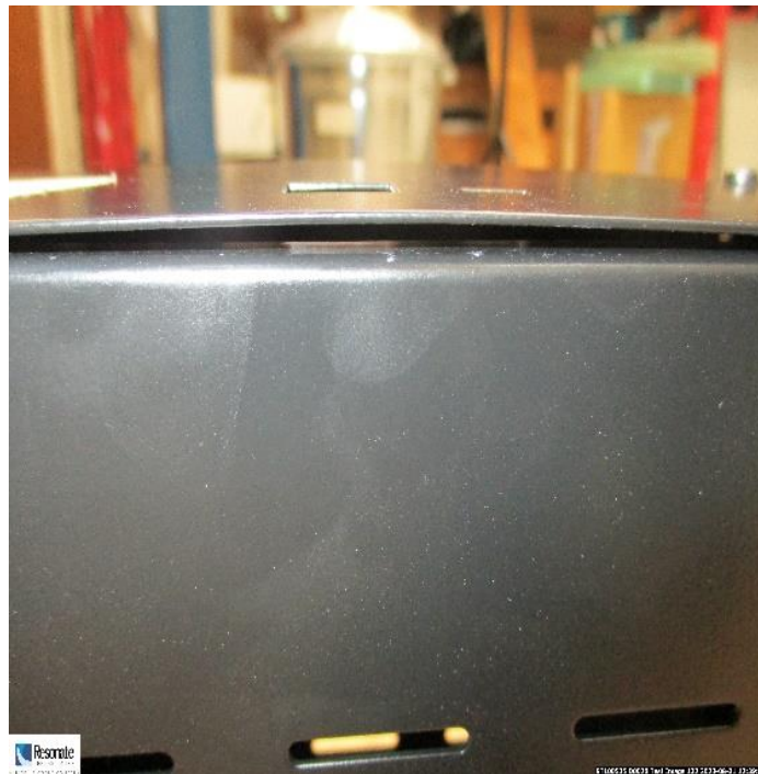
Figure 15: Observation after drop 16, edge bowing outwards
