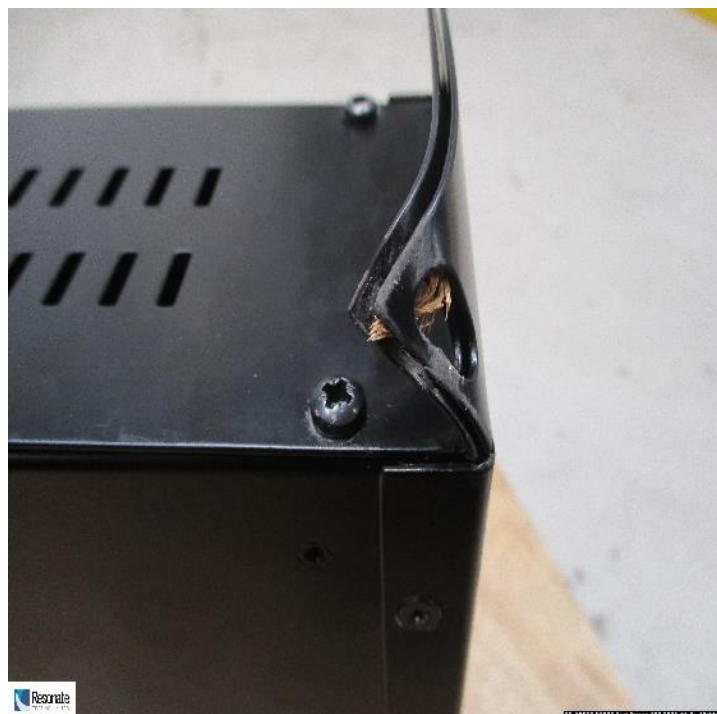
Figure 12: Observation after drop 10, corner of transit case front plate bent further
