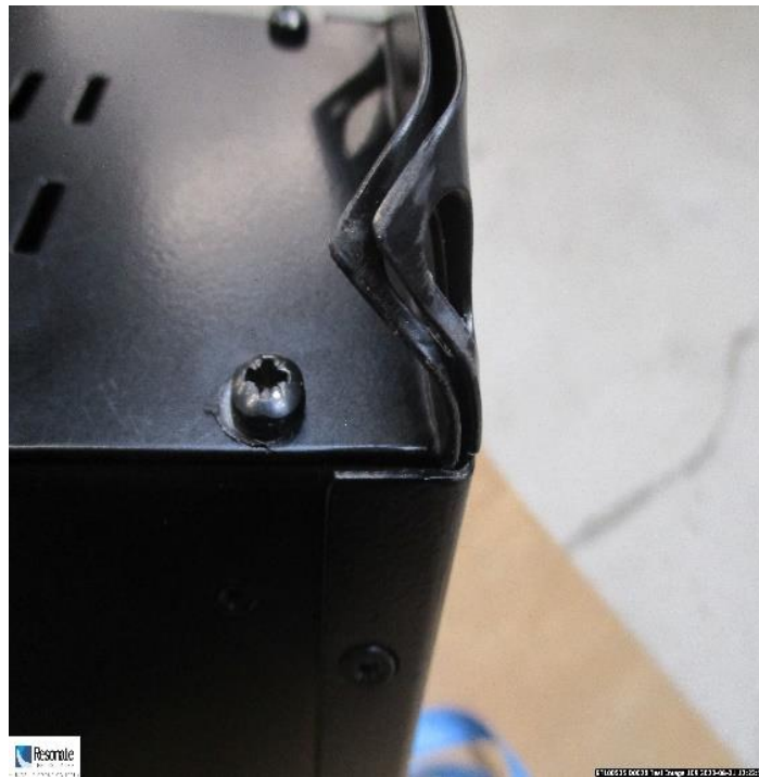
Figure 13: Observation after drop 13, corner of transit case front plate bent further
