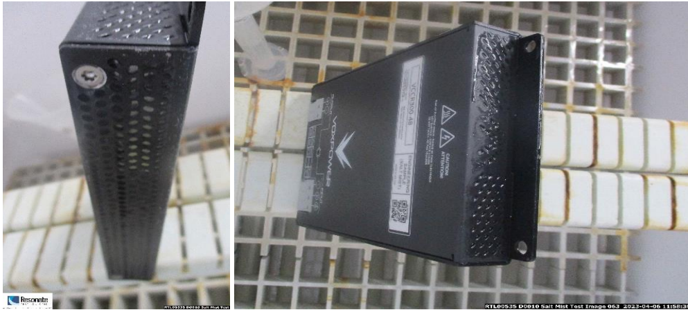
Figure 9: VCCR300-48 after 48-hour test
