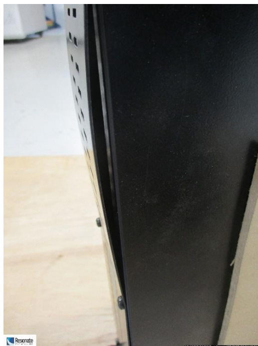
Figure 14: Observation after drop 15, bowing of edge
