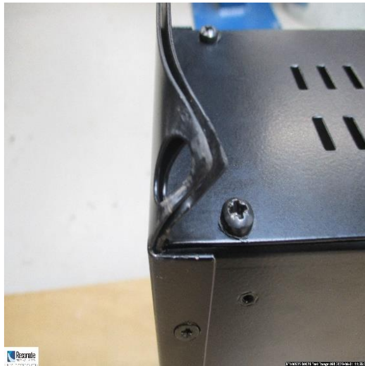
Figure 11: Observation after drop 9, corner of transit case front plate bent further
