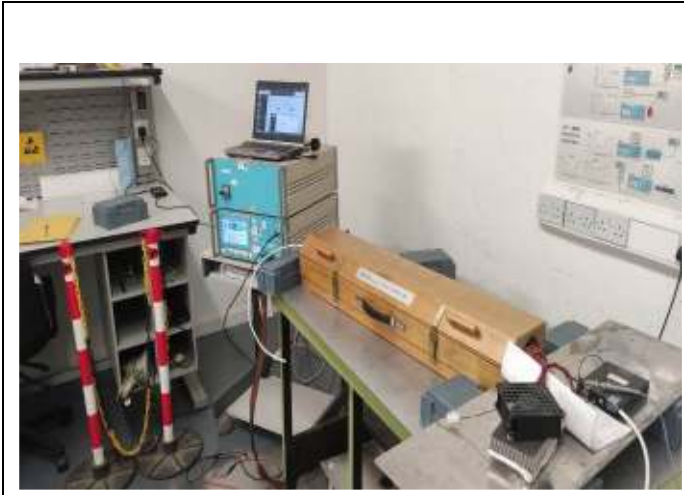
Figure 5: Fast Transient Test Set Up
