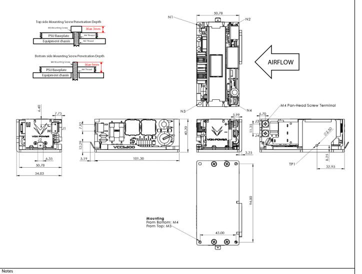
1. Top Side mounting screws are obstructed by components in some areas. M3 Hex socket screws should be used to allow angled access for tightening with a 2.5mm hex ball screwdriver. Care should be taken to ensure components are not damaged while tightening.
