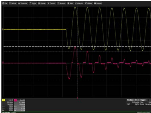
Figure 18: iMP8-3W0-3W0-30-A Inrush Current V_{IN} = 264 \text{ Vac} , No load Ch 1: AC Mains Ch 2: I_{IN}
