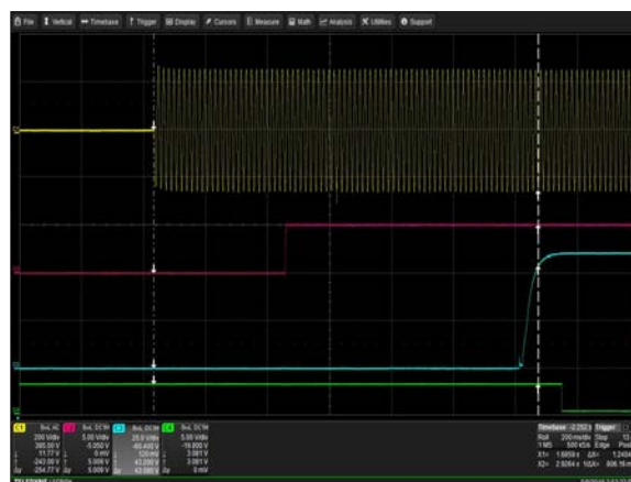
Figure 13: iMP8-3W0-3W0-30-A Turn-on Delay via AC mains
