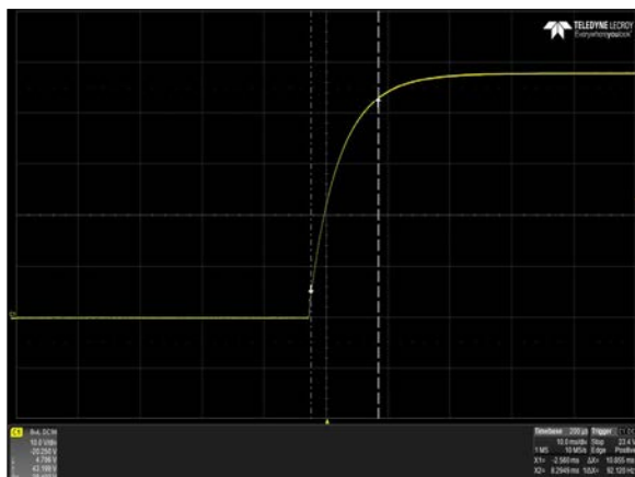
Figure 32: iMP4-1W0-00-A Output Voltage Startup Characteristic Load: I_O = 4\text{ A} , V_{IN} = 230\text{ Vac} Ch 1: V_O
