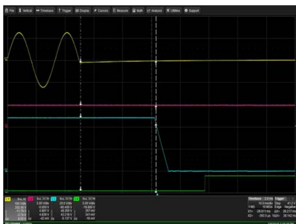
Figure 16: iMP8-3W0-3W0-30-A Hold Up Time
