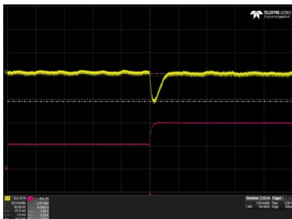
Figure 39: iMP4-2W0-00-A Transient Response – V_O Deviation 25% to 50% load change, 1 \text{ A}/\mu\text{s} slew rate, V_{IN} = 230 \text{ Vac} Ch 1: V_O Ch 2: I_O
