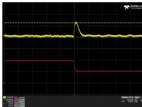
Figure 40: iMP4-2W0-00-A Transient Response – V_O Deviation 25% to 50% load change, 1 \text{ A}/\mu\text{s} slew rate, V_{IN} = 230 \text{ Vac} Ch 1: V_O Ch 2: I_O
