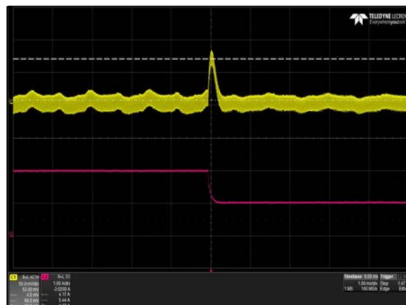
Figure 35: iMP4-1W0-00-A Transient Response – V_O Deviation 25% to 50% load change, 1\text{ A}/\mu\text{S} slew rate, V_{IN} = 230\text{ Vac} Ch 1: V_O Ch 2: I_O
