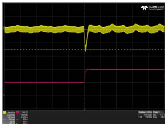
Figure 34: iMP4-1W0-00-A Transient Response – V_O Deviation 25% to 50% load change, 1\text{ A}/\mu\text{S} slew rate, V_{IN} = 230\text{ Vac} Ch 1: V_O Ch 2: I_O
