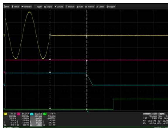
Figure 17: iMP8-3W0-3W0-30-A Hold Up Time
