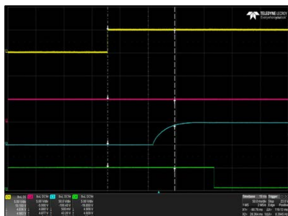
Figure 5: IMP4-3W0-2W0-30-A Turn-on Delay via Global Inhibit
