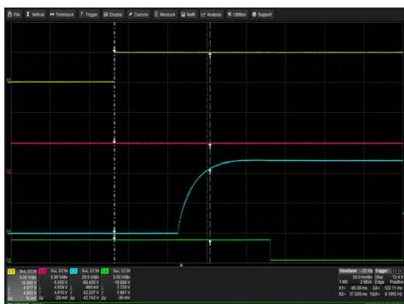
Figure 14: iMP8-3W0-3W0-30-A Turn-on Delay via Global Inhibit
