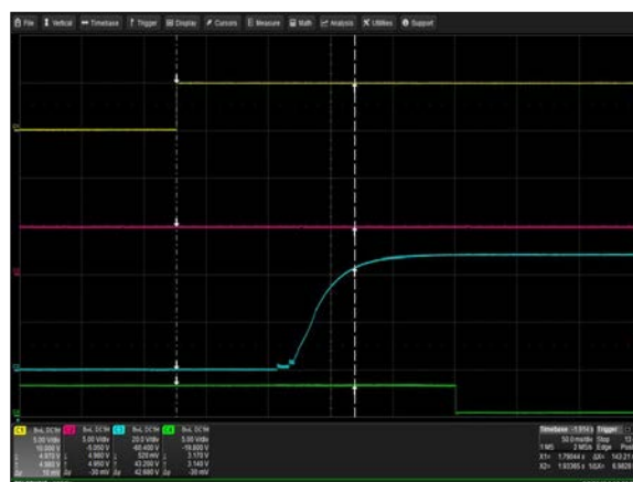
Figure 15: iMP8-3W0-3W0-30-A Turn-on Delay via Global Inhibit
