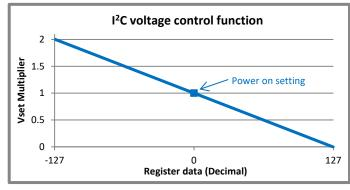
Example 1: OP1, Vset = 5V, Vadjust = 2V, I<sup>2</sup>C address = 20h, Voltage adjust register = F8h Use equation 2 to find the required data: 116.27\*(1-(2/5)) = +70Set sign bit (Bit 8 =1 for positive numbers, 0 for negative numbers): +70 => 198 (C6h) Equation 1 will give the quantized setting: Vout = 5\*(1-(70/116.27)) = 1.989VSend the following data over the I<sup>2</sup>C bus:
