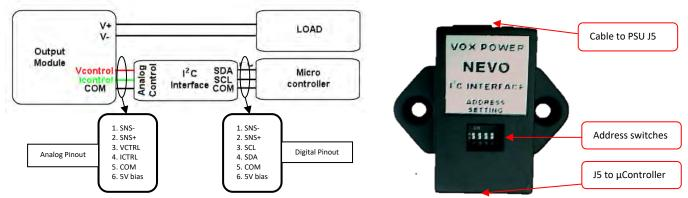
The output voltage and current limit can then be controlled in +/-127 steps that are programmed through the l<sup>2</sup>C interface. Careful consideration must be given to system grounding as the interface is <u>not</u> isolated and must be referenced to the COM pin on J5. Incorrect system grounding may cause damage to the unit. Adhere to the same precautions as for "Local bias supply" detailed on page 16 of the user manual or contact Vox Power for assistance.
