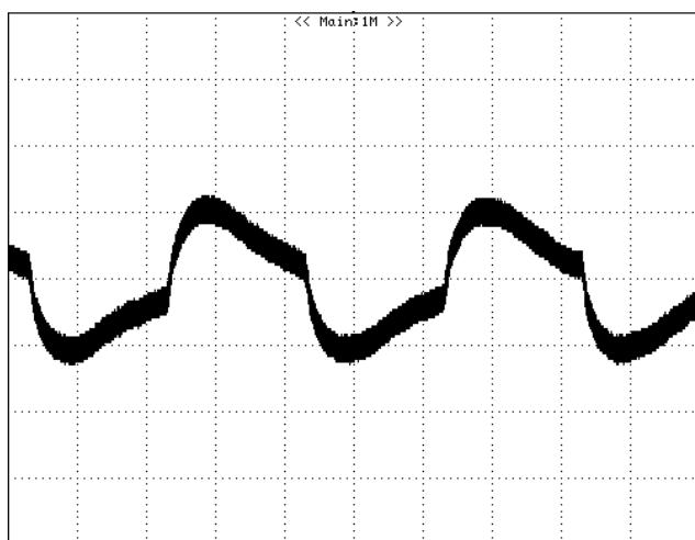
**Figure 3:** Dynamic response to load step 7.5A~11.25A with 0.1A/uS slew rate at 48Vin
