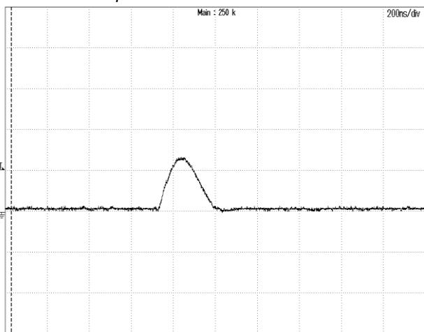
**Figure 11:** Inrush current @ Vin=48V CH1:lin, 2A/div,
