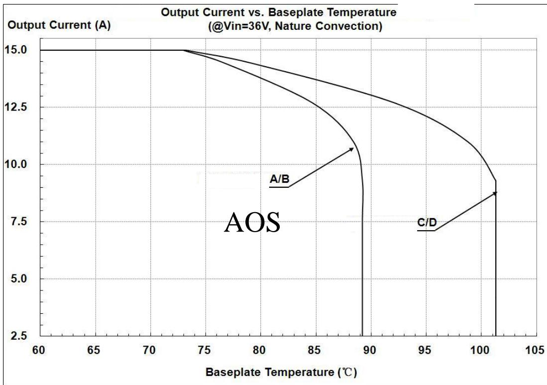
Figure 24: Output Current vs. Base Table temperature @ Vin=36V
