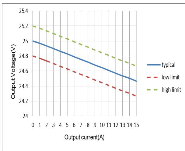
**Figure 9:** Output voltage vs. Output current
