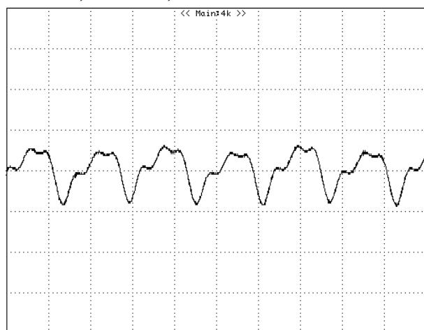
**Figure 5:** Output ripple & noise at 48Vin, 15A lout
