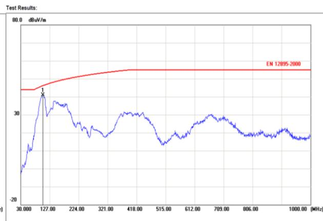
**Figure 15:** test result(Horizontal)
