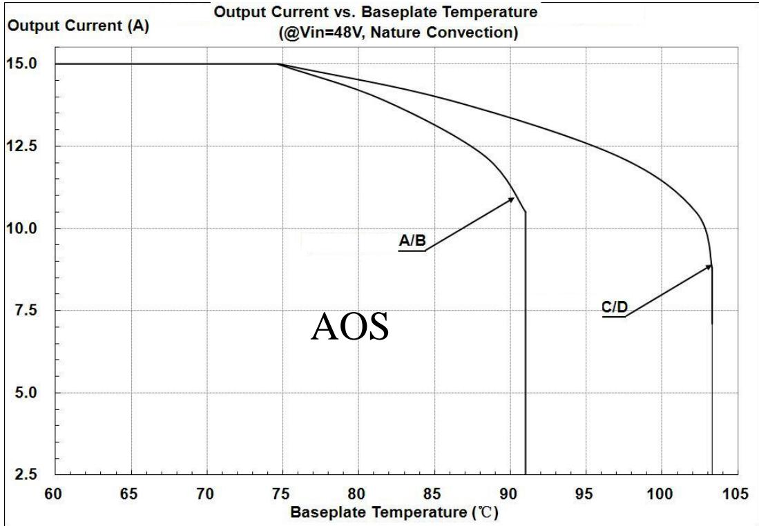
Figure 25: Output Current vs. Base Table temperature @ Vin=48V
