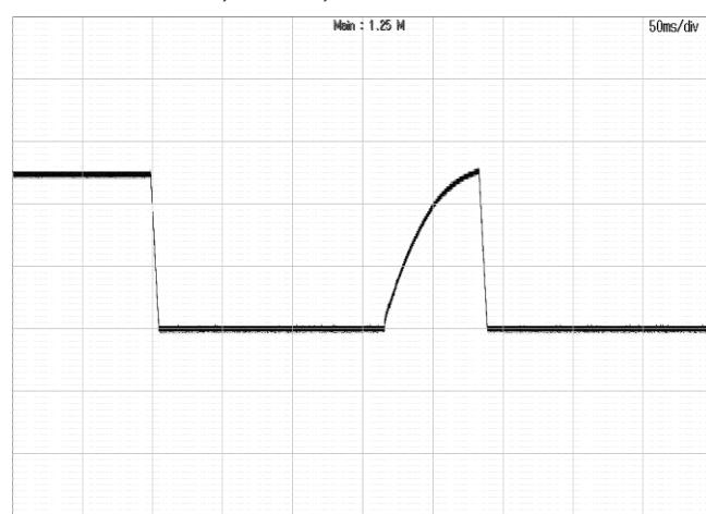
**Figure 6:** Output over voltage protection at 48Vin, 7.5A lout
