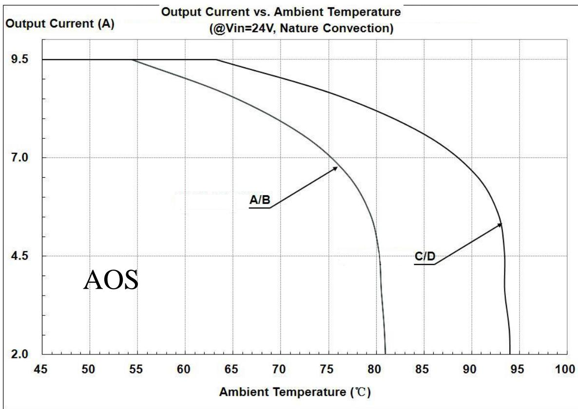
**Figure 17:** Output Current vs. Ambient temperature @ Vin=24V
