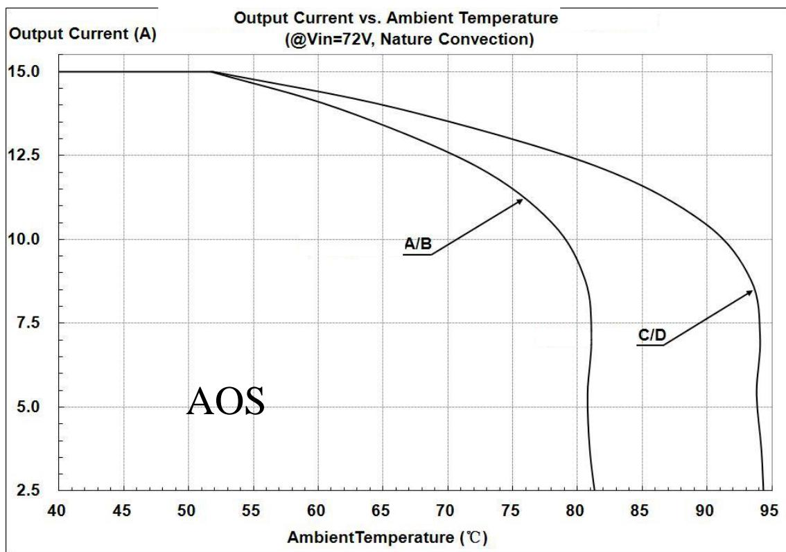
Figure 20: Output Current vs. Ambient temperature @ Vin=72V
