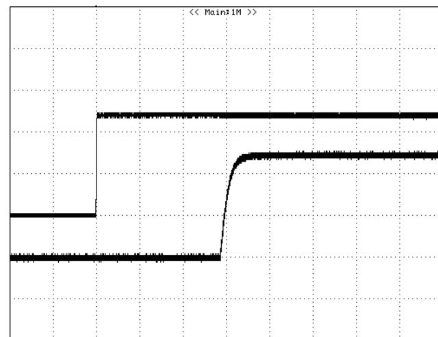
**Figure 4:** Vout start up with Vin on at 48Vin, 15A lout,
