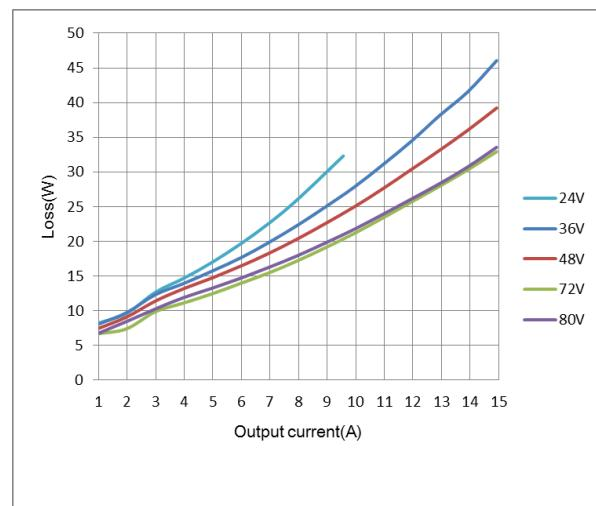
**Figure 2:** Loss vs. Output current
