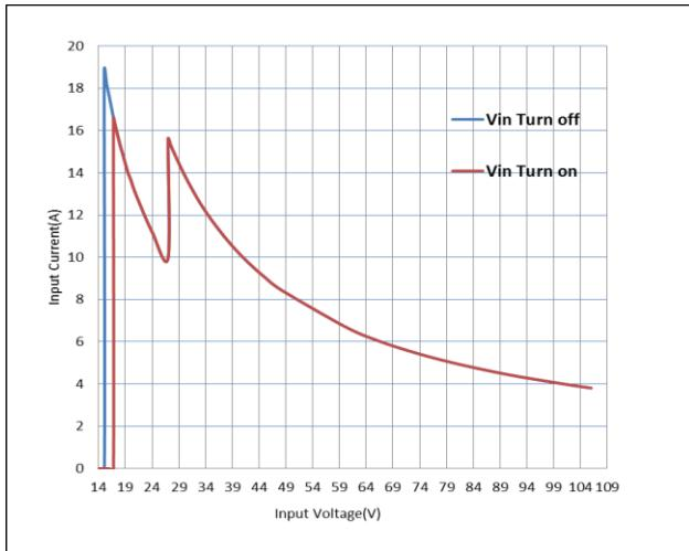
**Figure 7:** Input current vs. Input voltage
