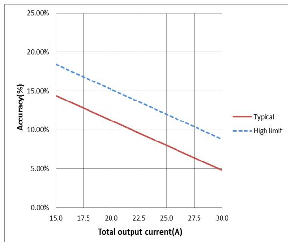
**Figure 10:** Current share accuracy vs. Total output current
