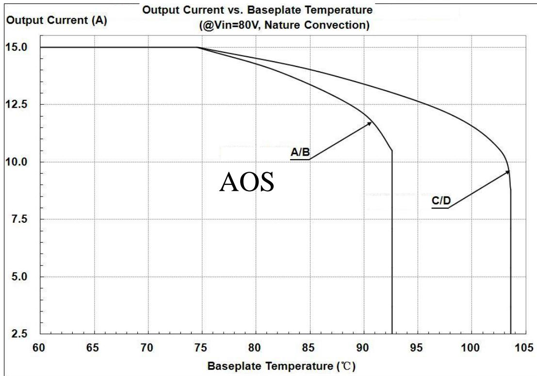
Figure 27: Output Current vs. Base Table temperature @  $V_{in}=80V$
