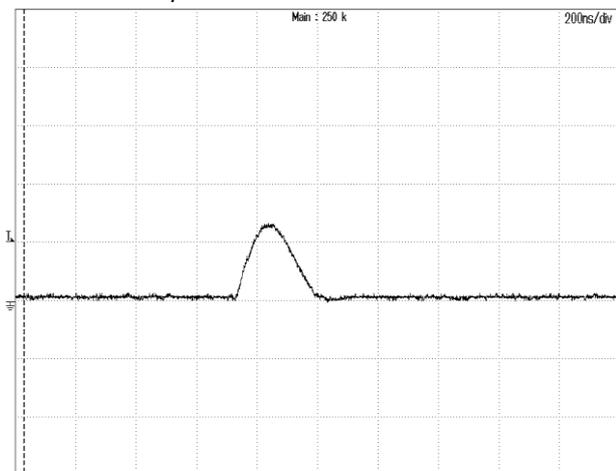
**Figure 11:** Inrush current @ Vin=48V
