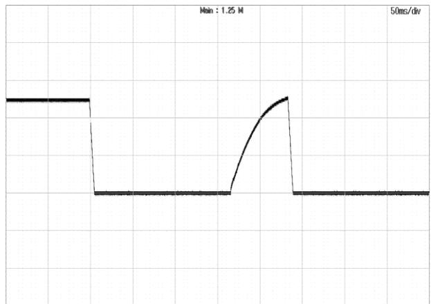
**Figure 6:** Output over voltage protection at 48Vin, 6.25A lout
