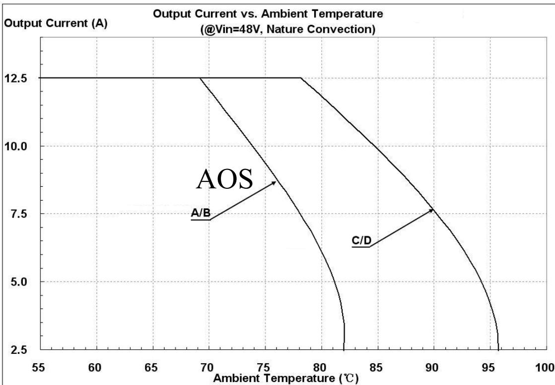
Figure 19: Output Current vs. Ambient temperature @ Vin=48V
