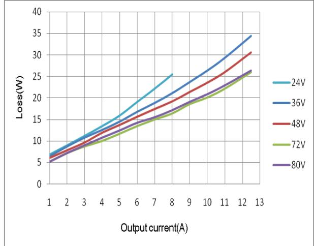
@ **Figure 2:** Loss vs. Output current
