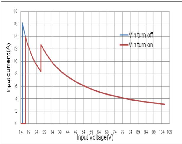
**Figure 7:** Input current vs. Input voltage
