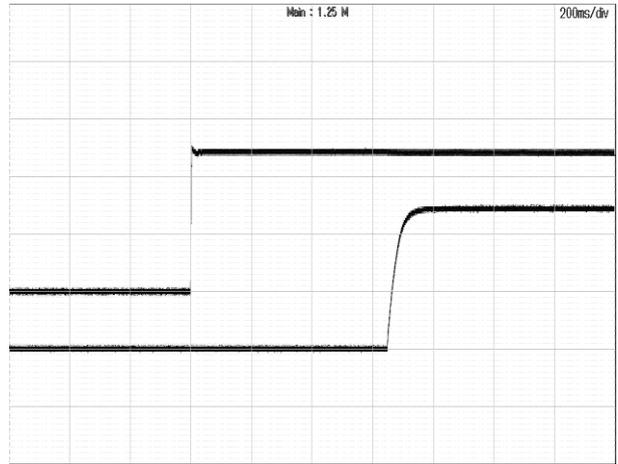
**Figure 4:** Vout start up with Vin on at 48Vin, 12.5A lout,
