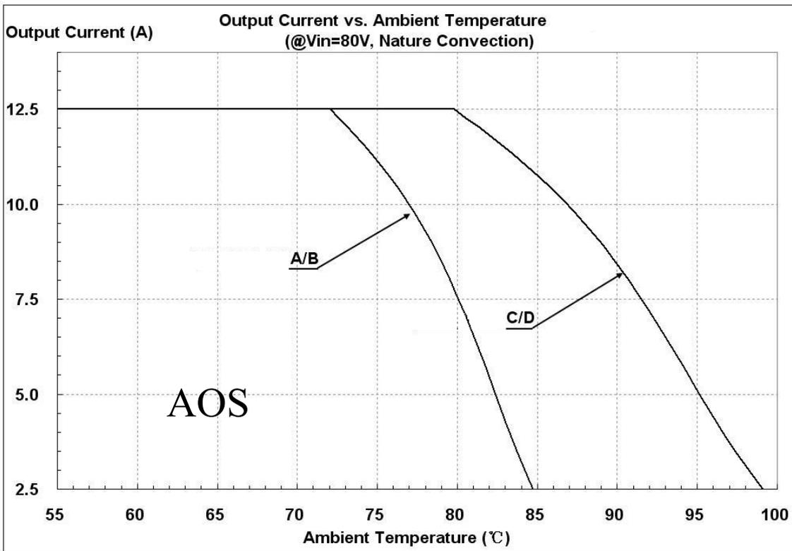
Figure 21: Output Current vs. Ambient temperature @ Vin=80V
