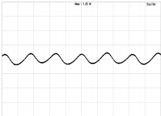
**Figure 5:** Output ripple & noise at 48Vin, 12.5A lout
