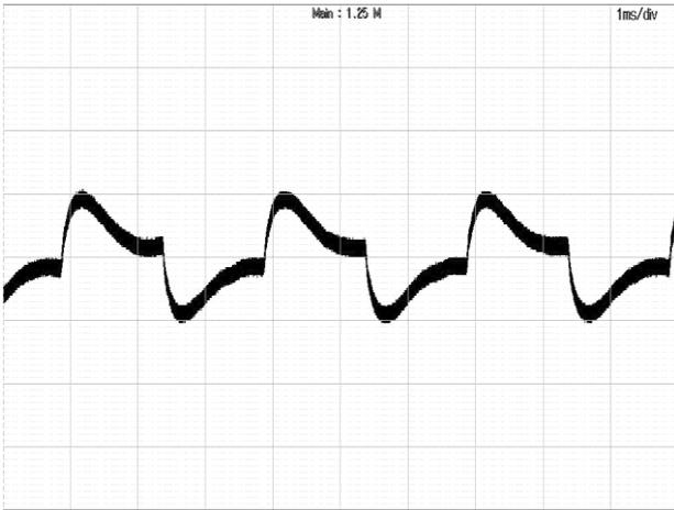
**Figure 3:** Dynamic response to load step 6.25A~9.375A
