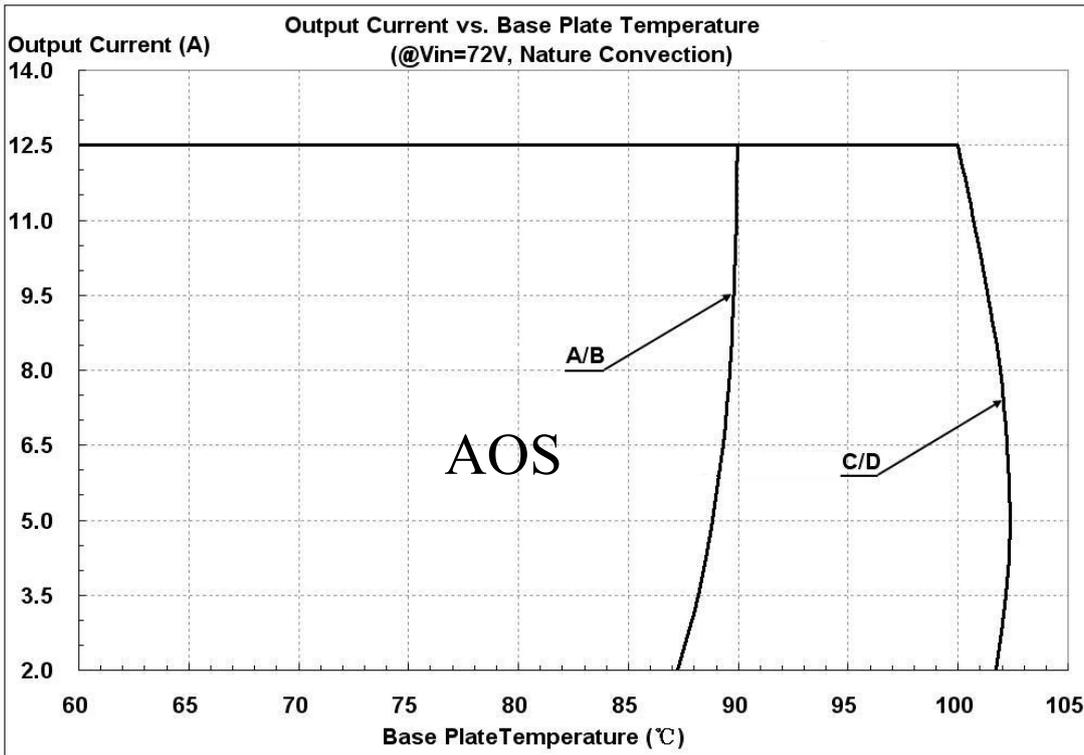
Figure 26: Output Current vs. Base Table temperature @ Vin=72V
