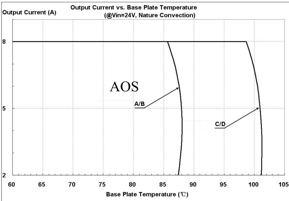
Figure 23: Output Current vs. Base Table temperature @ Vin=24V
