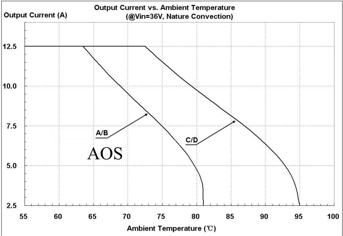
Figure 18: Output Current vs. Ambient temperature @ Vin=36V
