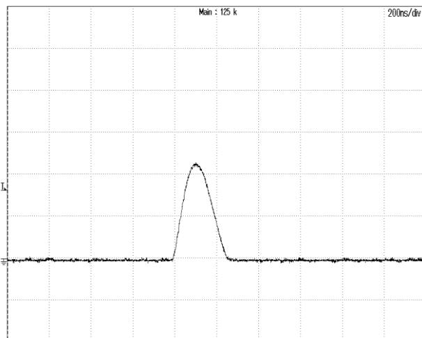
**Figure 11:** Inrush current @ Vin=72V
