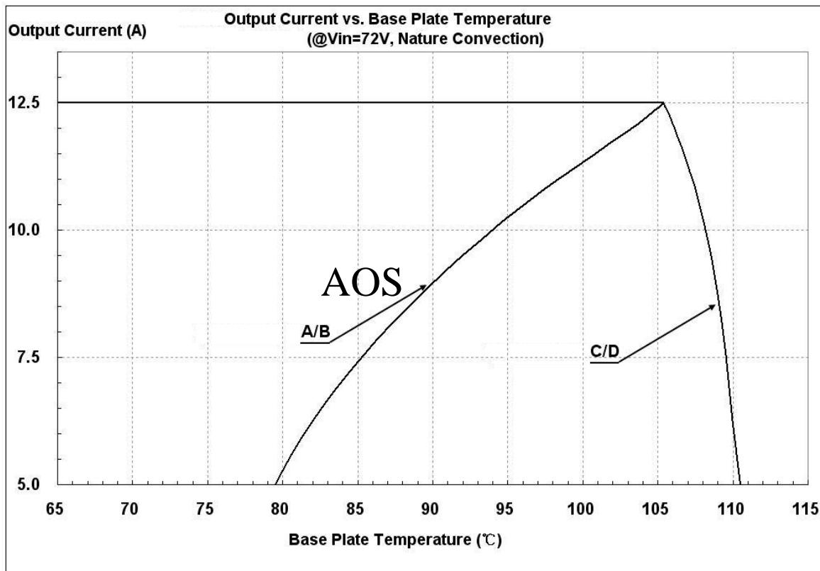
Figure 22: Output Power vs. base plate temperature @ $V_{in}=72V$
