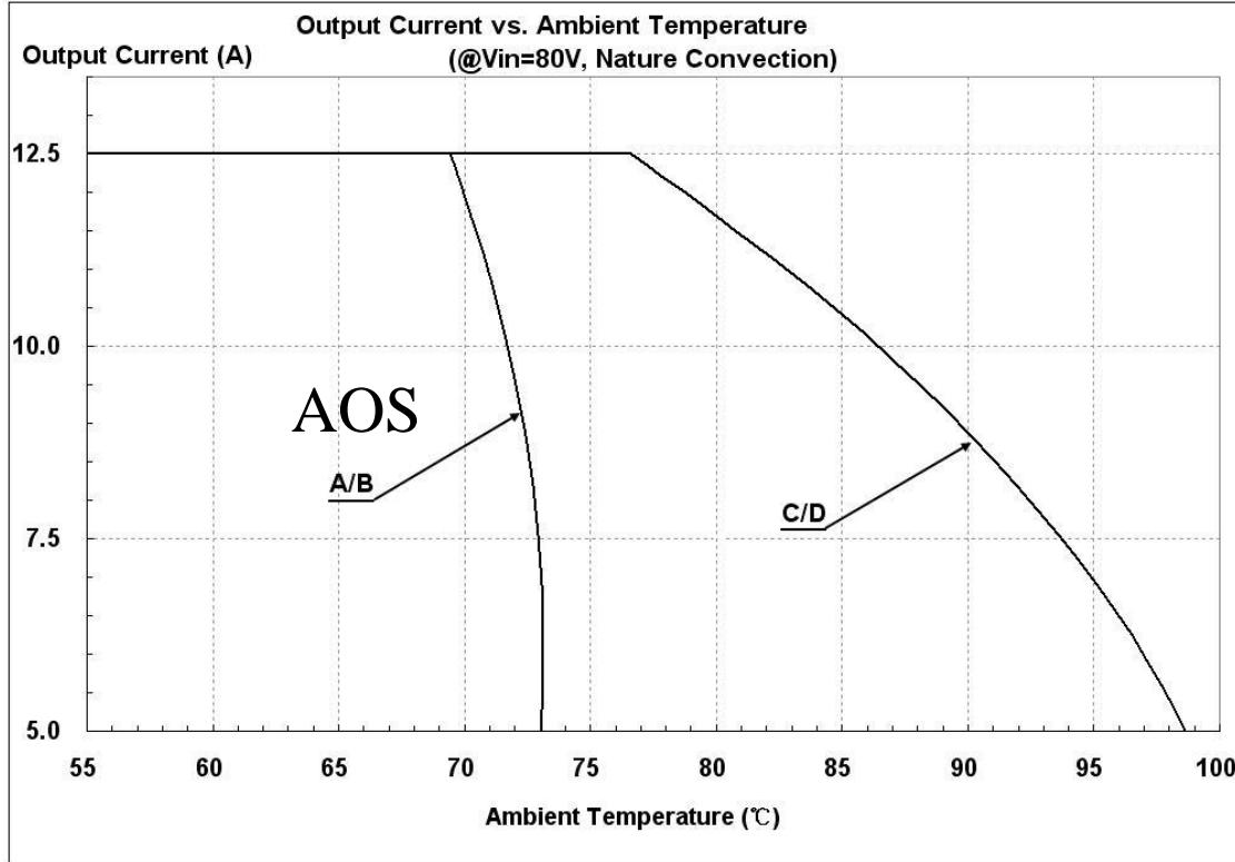
Figure 19: Output Current vs. ambient temperature @ $V_{in}=80V$
