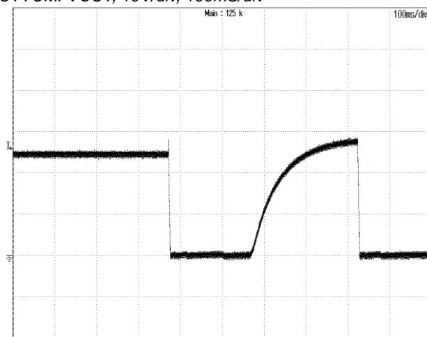
**Figure 10:** Output over voltage protection at 72Vin, 24A lout
