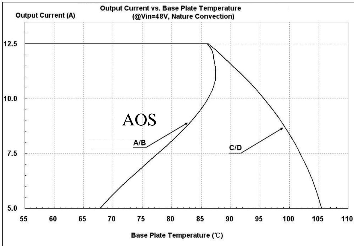
Figure 21: Output Power vs. base plate temperature @Vin=48V
