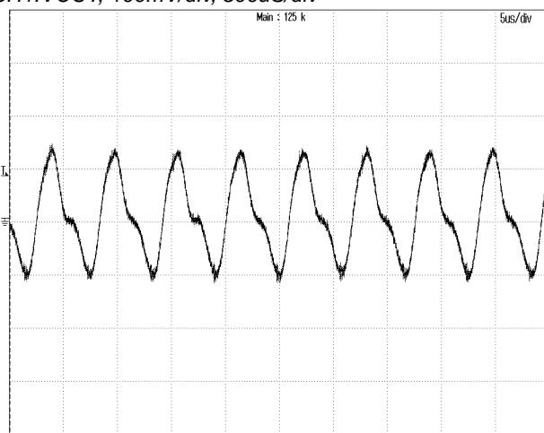
**Figure 9:** Output ripple & noise at 72Vin, 24A lout
