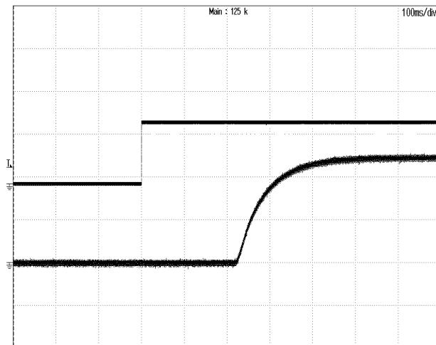
**Figure 8:** Vout start up with Enable on at 72Vin, 12.5A lout,
