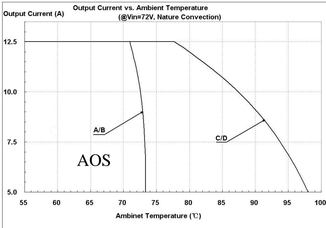
Figure 18: Output Current vs. ambient temperature @ $V_{in}=72V$
