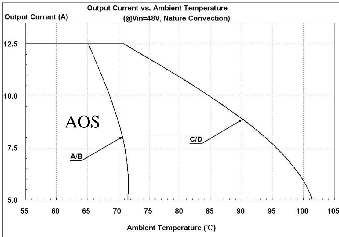
*Figure 17: Output Current vs. ambient temperature @Vin=48V*
