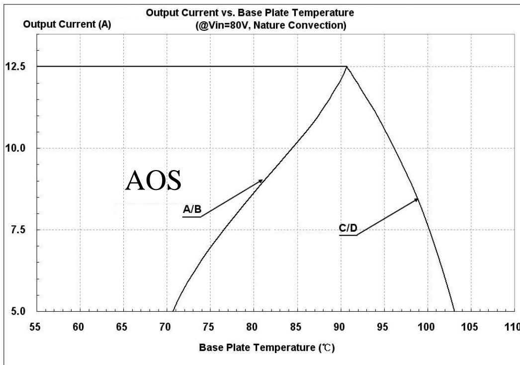
Figure 23: Output Power vs. base plate temperature @ $V_{in}=80V$
