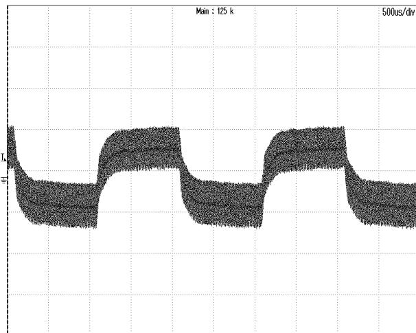
**Figure 7:** Dynamic response to load step 6.25A~9.375A with 0.1A/uS slew rate at 72Vin
