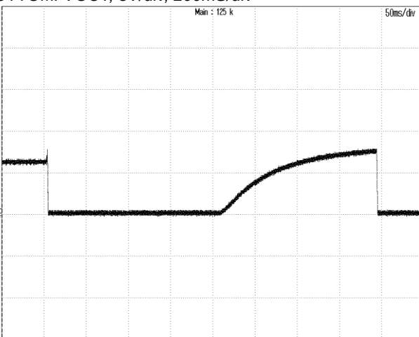
Figure 6: Output over voltage protection at 72Vin, 24A Iout CH1:VOUT, 10V/div, 50mS/div
