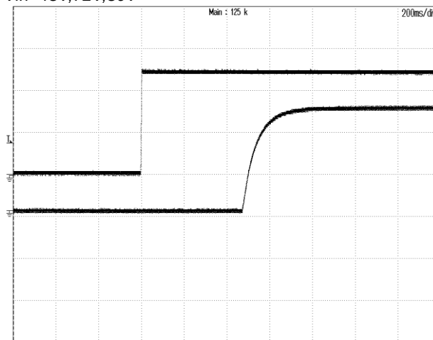
Figure 4: Vout start up with Vin on at 72Vin,24A Iout, TOP:VIN, 20V/div, 200mS/div BOTTOM: VOUT, 5V/div, 200mS/div
