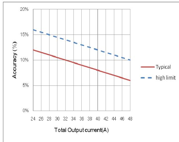
Figure 14: Current share accuracy vs. Total output current
