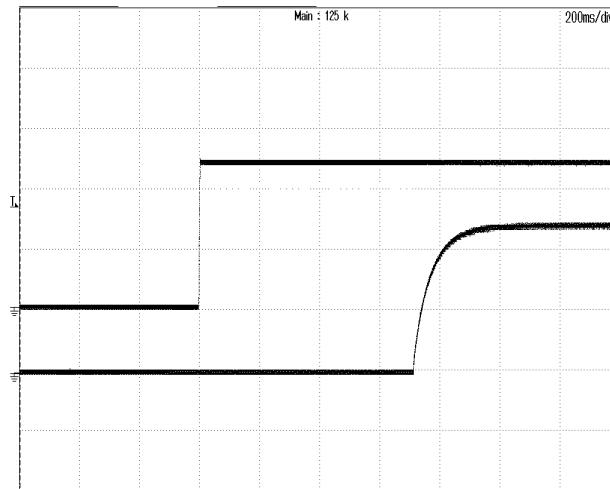
**Figure 6:** Vout start up with Vin on at 48Vin, 24A lout,
