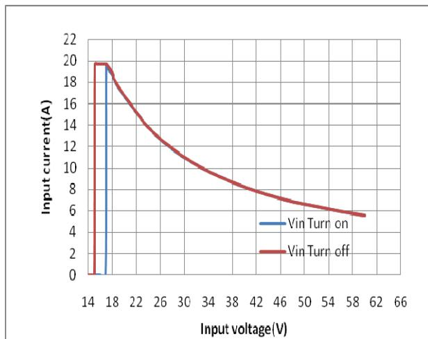
Figure 11: Input current vs. Input voltage
