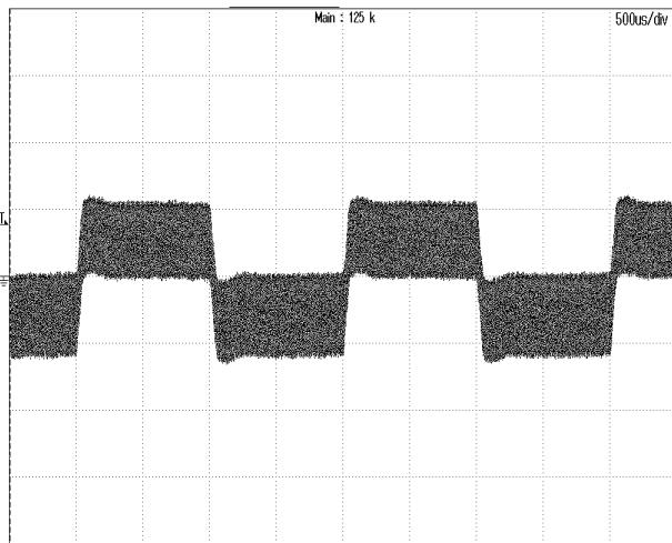
**Figure 5:** Dynamic response to load step 12A~18A with 0.1A/uS slew rate at 48Vin
