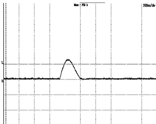
Figure 15: Inrush current @ Vin=48V
