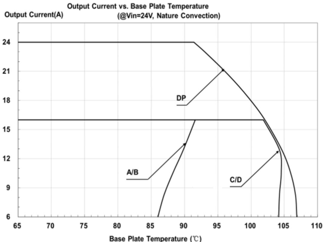
Figure 25: Output Current vs. Base Plate temperature @Vin=24V
