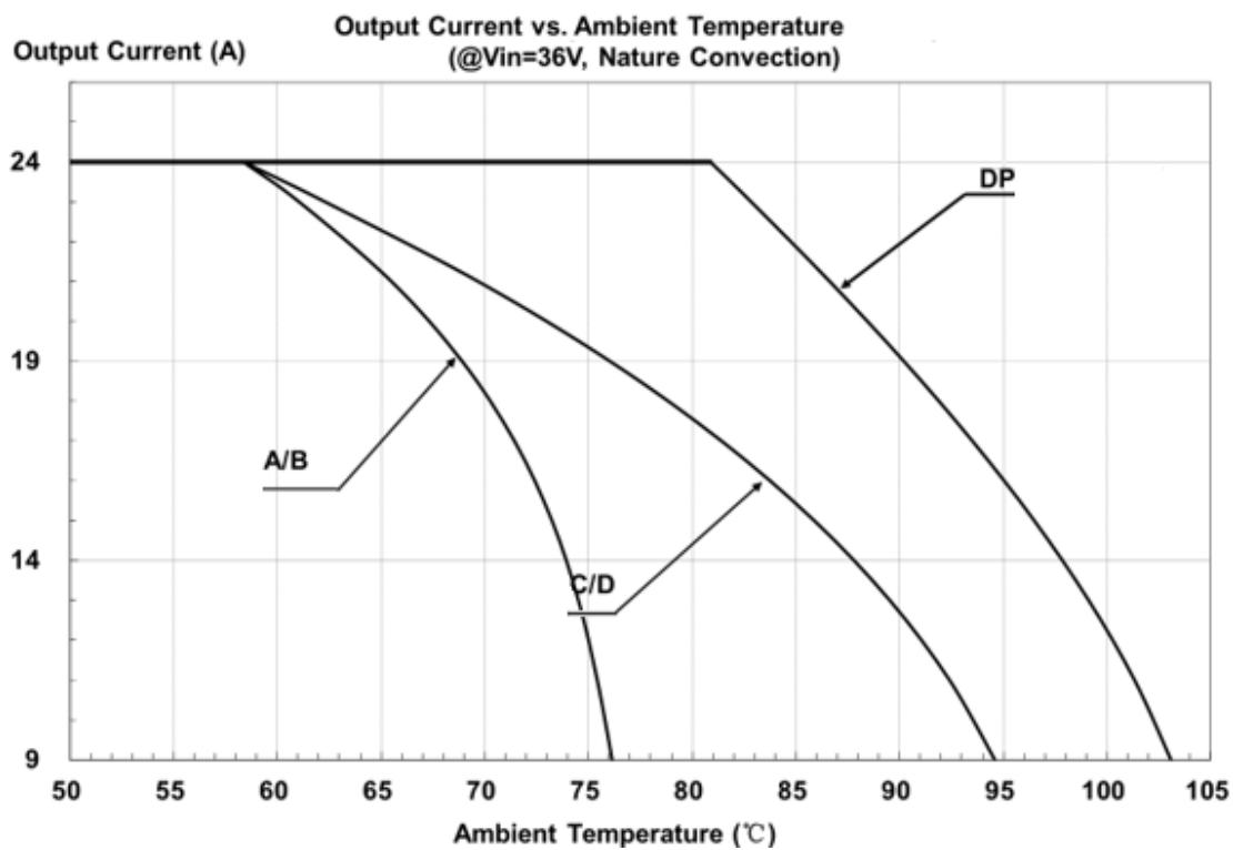
Figure 22: Output Current vs. Ambient temperature @ Vin=36V
