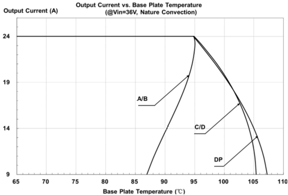
Figure 26: Output Current vs. Base Table temperature @ Vin=36V
