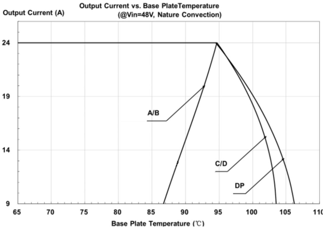
Figure 27: Output Current vs. Base Table temperature @ Vin=48V
