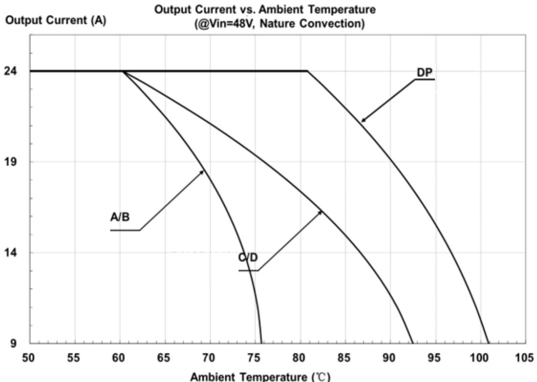
Figure 23: Output Current vs. Ambient temperature @ Vin=48V
