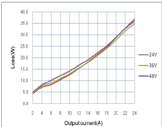
**Figure 4:** Loss vs. Output current
