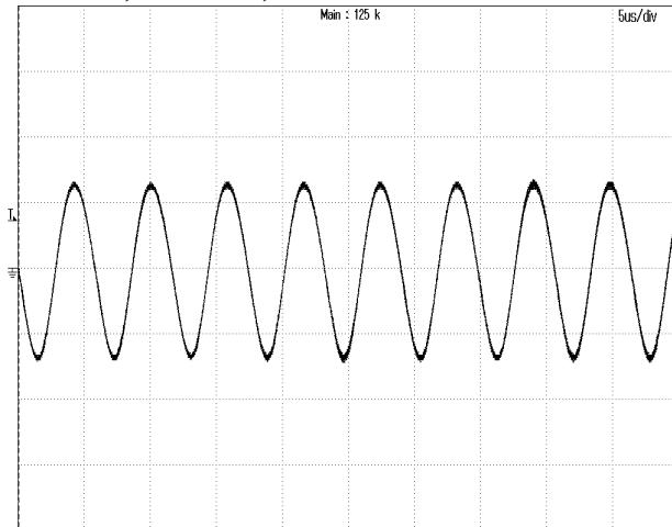
**Figure 7:** Output ripple & noise at 48Vin, 24A lout
