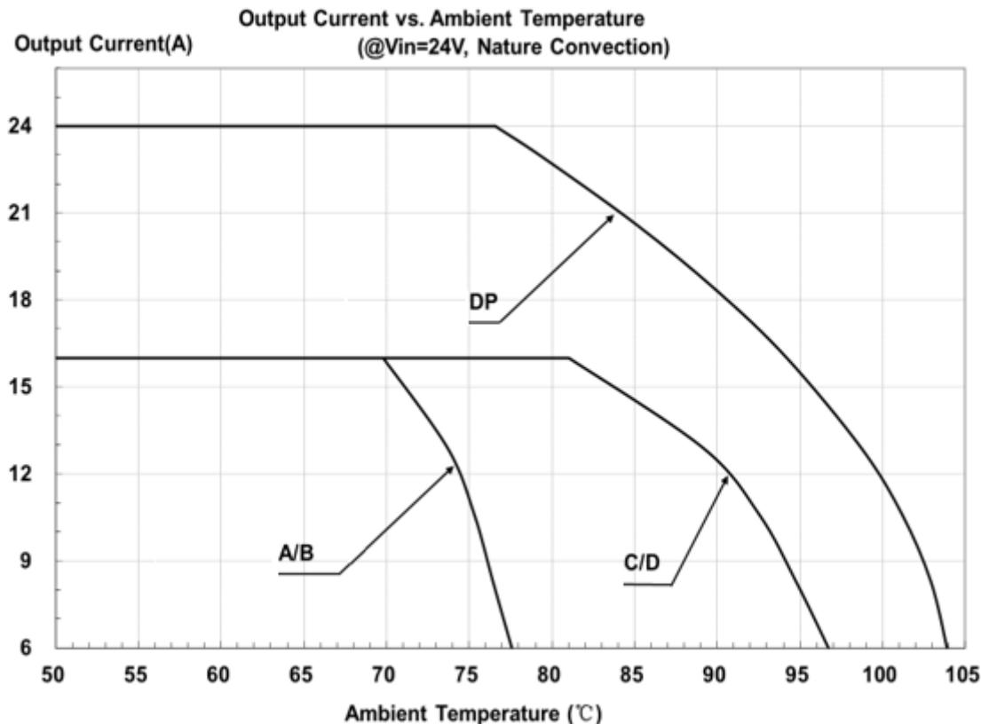
Figure 21: Output Current vs. Ambient temperature @ Vin=24V
