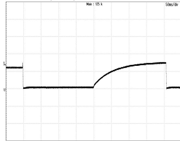
**Figure 8:** Output over voltage protection at 48Vin, 24A lout
