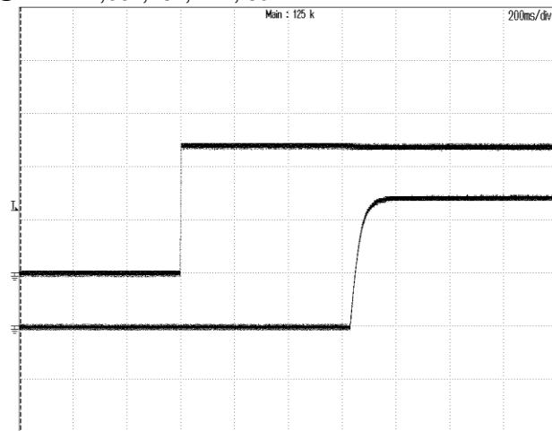
**Figure 4:** Vout start up with Vin on at 48Vin, 24A lout,
