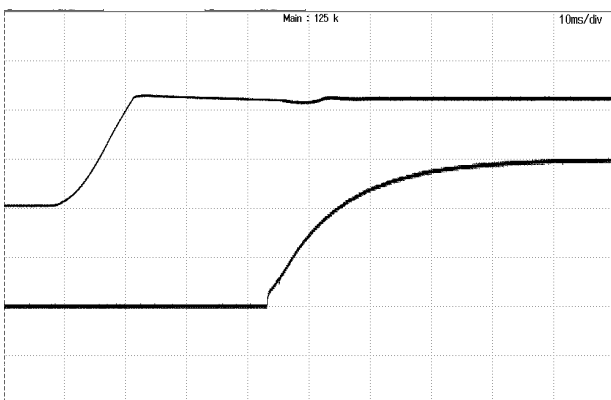
Figure 5: Turn-on transient at zero load current (20ms/div). Top Trace: Vout; 5V/div; Bottom Trace: input voltage; 50V/div.
