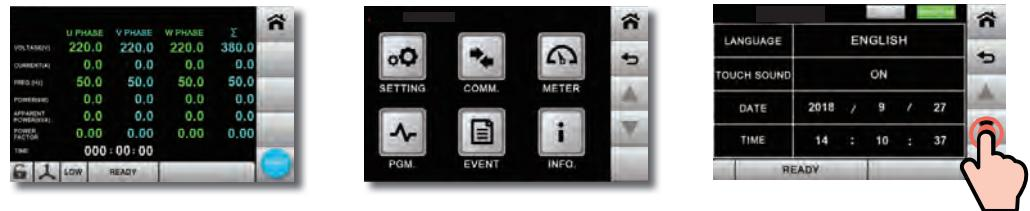
The VPV + series employs 7" touch screen to provide intuitive and easy-to-use control and display. Users can quickly access output settings and measurements, including voltage, current, frequency, real power, apparent power, PF and sum of each phase's parameters. Complex sequences and system configurations can also be easily done via the touch screen.
