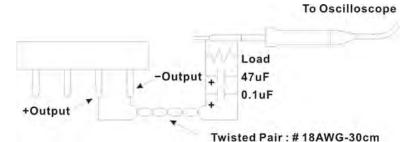
A 30cm twisted pair of no.18 AWG copper wire is connected to a 47uF and 0.1uF capacitor of proper polarity and voltage rating. The oscilloscope probe ground led should connect right to the ground ring of the probe and be as short as possible. The oscilloscope bandwidth should be at 20MHz and connected to AC ground.
